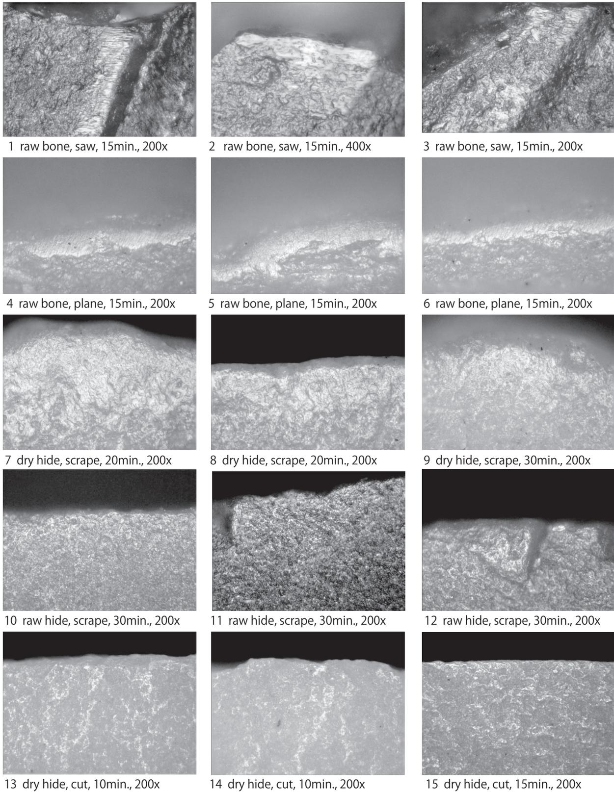
Fig.2 Use-wear polishes on experimental lithic tools.
