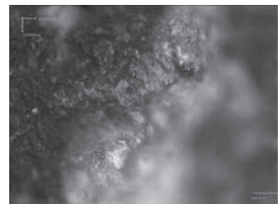
8: B type polish with vertical striation (x400)
